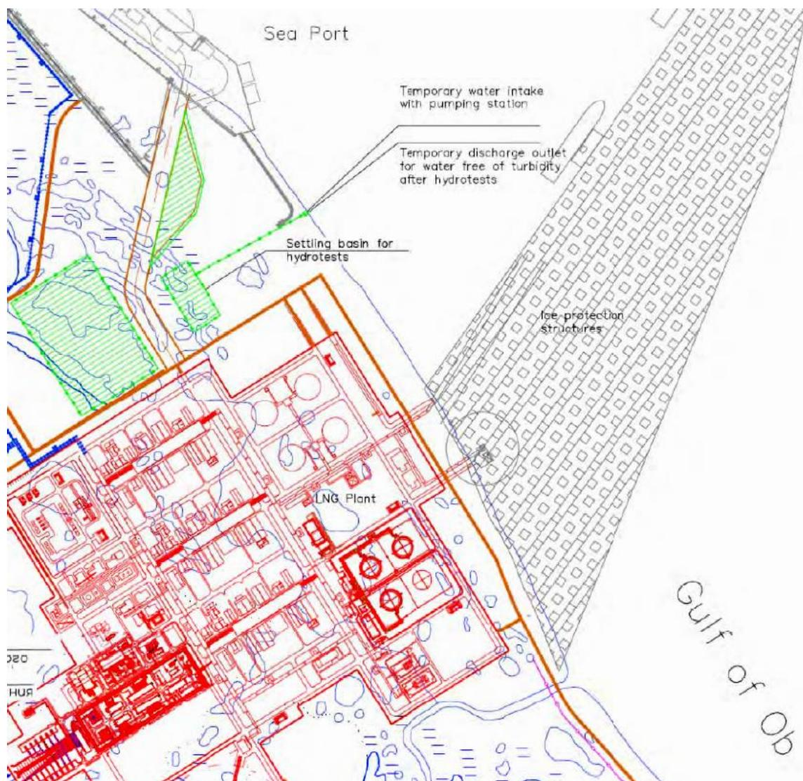
**Figure 9.4.3: Arrangement of temporary water intake and settling basin during hydrotesting**
